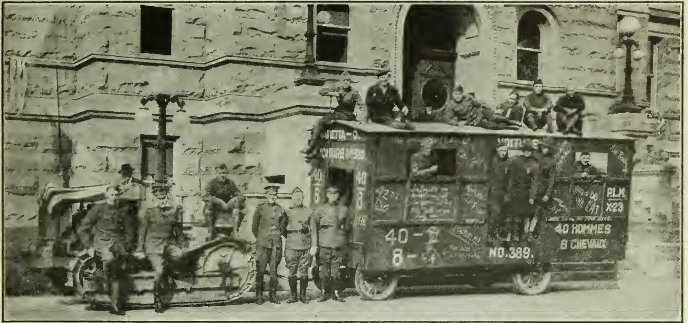
Marietta (Ohio) Voiture of the Forty and Eight faithfully reproduced everything but the flat wheels when it built this French boxcar for an Armistice Day parade. Ten men did the job in two evenings at a cost of $20 for lumber. The boxcar is built in five pieces—two sides, two ends and a roof—and is mounted on a Ford chassis
